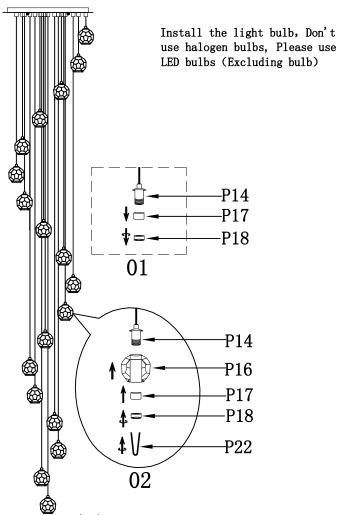
01. Unscrew the lamp holder ring (P18) counterclockwise, and then remove the iron tube (P17);
